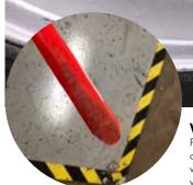
Why use something not designed to last? Plastic Scrappers are an alternative to using knifes and other sharp abrasive objects that can damage aluminum wheels while removing adhesive wheel weights but they wear quickly.
