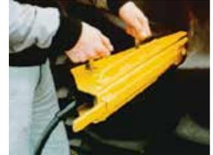
**Slide Hammer Bead Breaker- Manual Style Bead Breaker**
