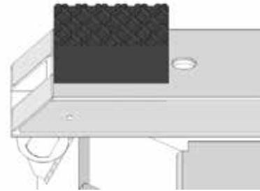
Clean the surface of the jacking point of the vehicle, so that there is no grease or oil to avoid possible slipping of the vehicle.
