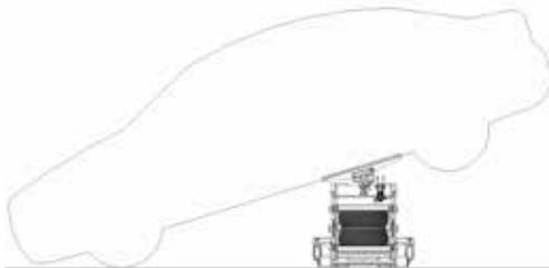
**miniLIFT can lift the vehicle from one end or the other. the minilift is NOT a full vehicle lift system on its own.**
